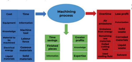
Illustration 1. Reliable and unreliable machining process
